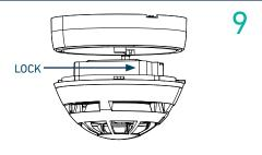
• Ensure you replace the battery cover as this forms part of the detectors anti-tamper protection and refit the detector locating it into the base twisting clockwise.
